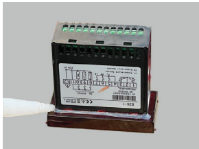
Figure 5: Apply silicone around the frame as shown.
